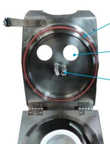
Lid gasket in silicone rubber PTFE encapsulated
